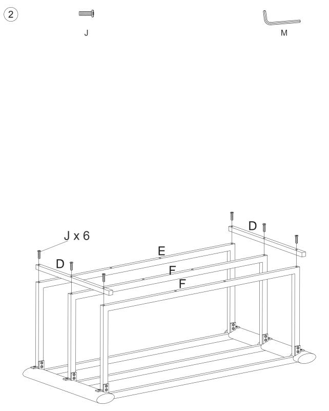
2. Fasten pillars (D) to the frames (E&F) with screws (J)
